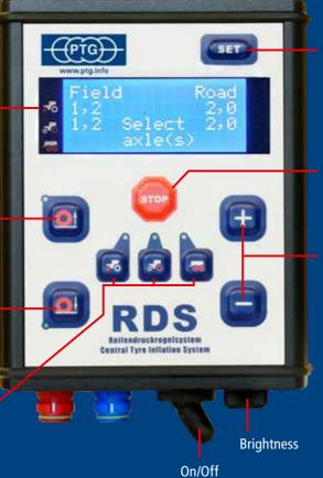
To adjust the set inflation pressures (permanent): press and hold
